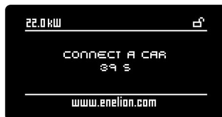
Chargers with Plug And Charge configuration only wait for the car to be connected. Once the cable is properly connected the charging process will start.
