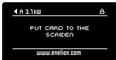
The active connector will switch over upon pressing the button located on the left under the display or automatically upon connecting or disconnecting the cable to the charger. During the switch the display will show a letter informing which connector the user interface has been switched to.
