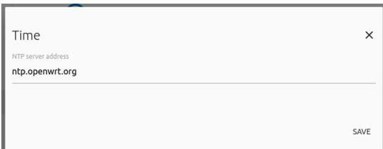
Fig. 20: NTP time synchronization server settings.
