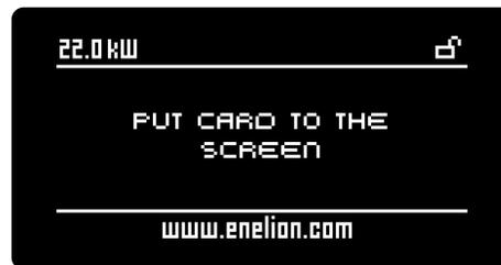
Once the card is verified correctly the charger will wait for the car to be connected. The timer located under the message shows time within which the user should connect the car in order to start the charging process. When the time elapses, you should place the card on the display again. When the car is correctly connected and the lock in the chargers equipped with sockets are locked, the charging process will begin.
